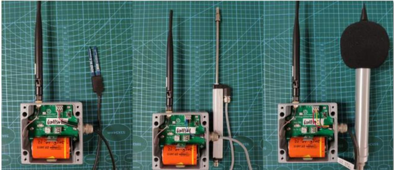
图. 电压支点连接传感器示意图(From left to right: EC-5 Soil Moisture in %, Displacement in mm, Noise Level in dB.)
