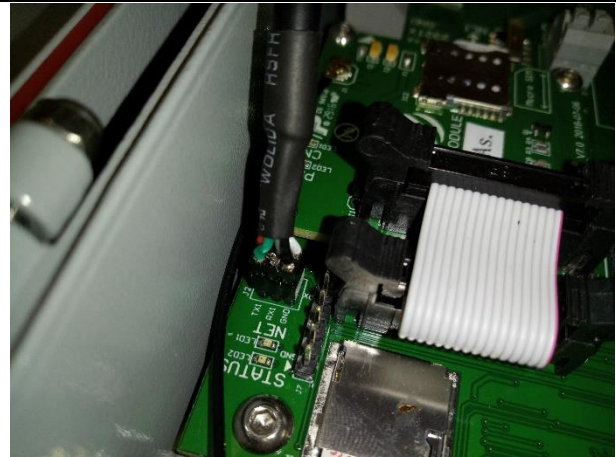
Figure. TTL to USB Connection.
