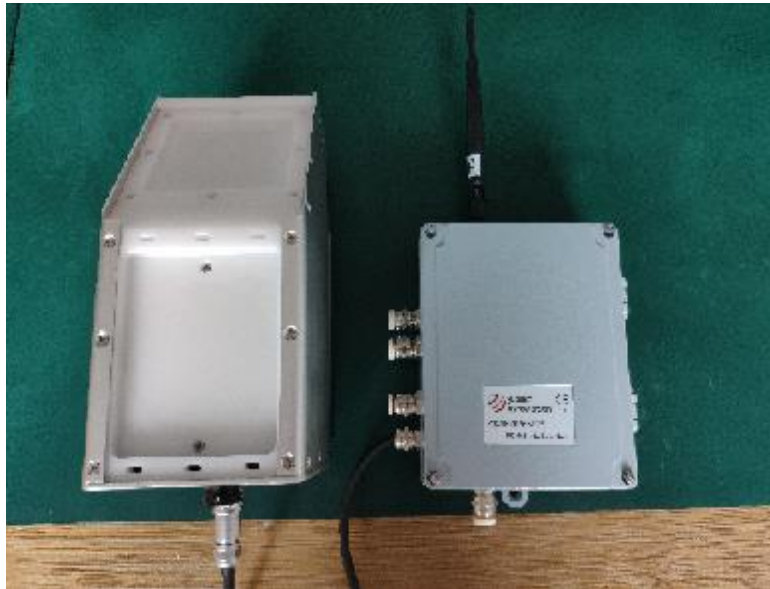
Figure. Radar Flow Meter Sensor Node.
