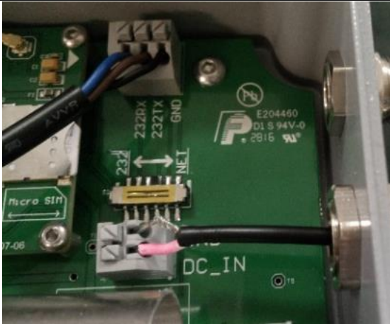
Figure. 110-240VAC to 12VDC@5A Adapter Connection.
