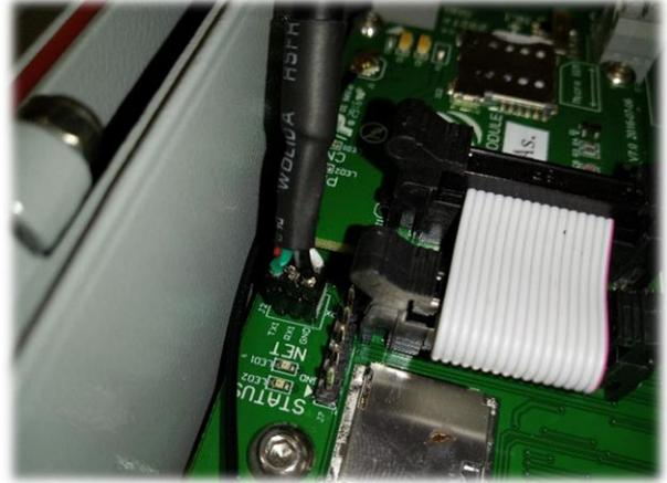
Figure. TTL to USB Connection.
