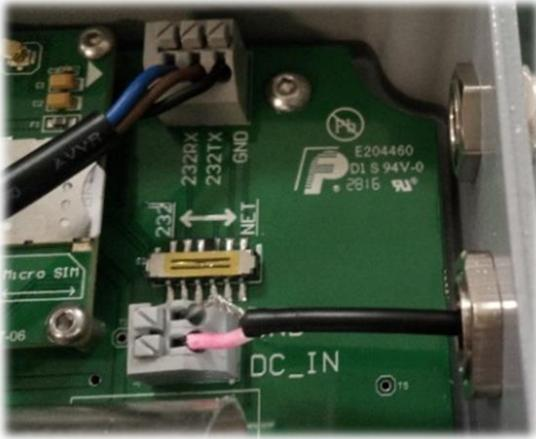
Figure. 110-240VAC to 12VDC@5A Adapter Connection.
