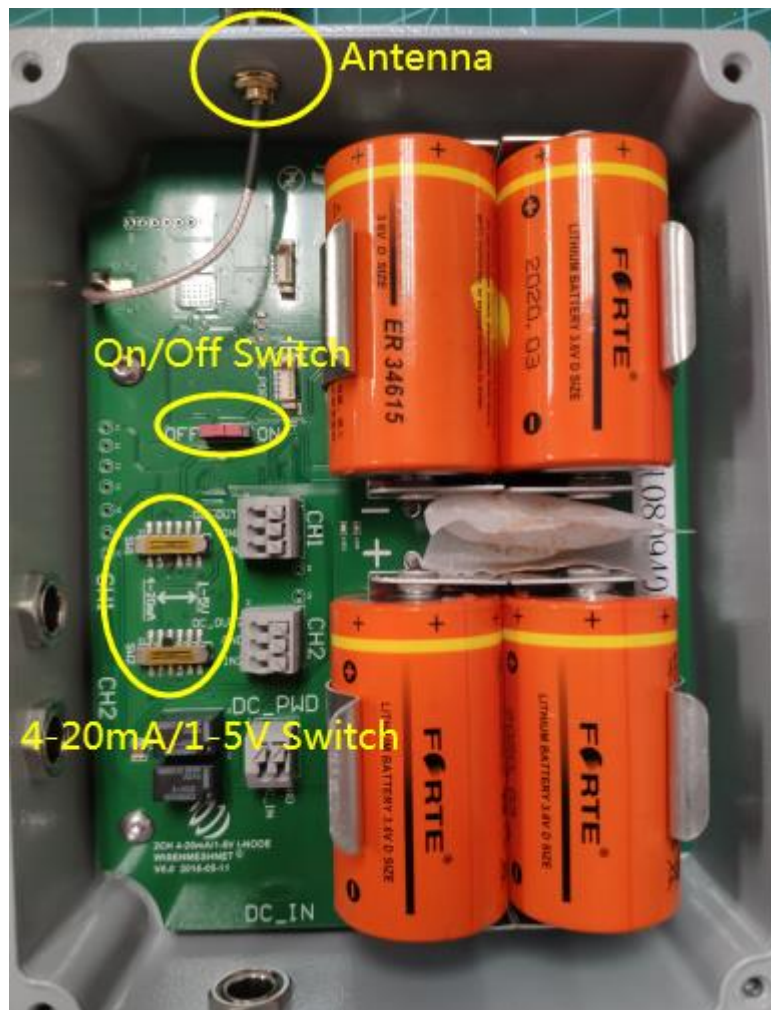
Figure 3. 2-Channel 4-20mA/1-5V Interface Node Internal Configuration Terminologies, where:
